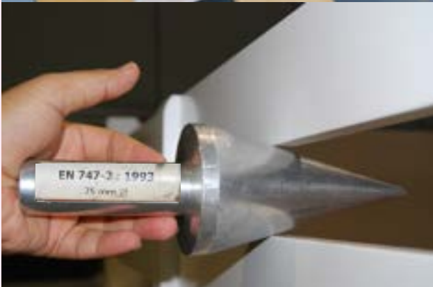
Cylindrical and conical test probes with diameters measuring 25, 60, 75 and 80 mm are used to assess the risk of entrapment in or between bed base and other structures
