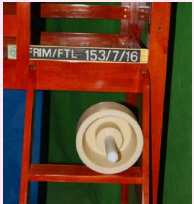
The head probe (circular device) should pass through the opening to reduce the risk of head entrapment
