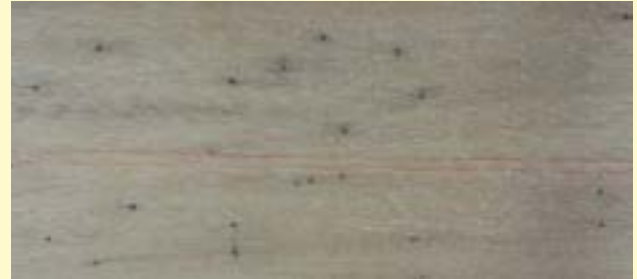
Small pin-holes are common characteristic of defect in cengal. The holes are caused by ambrosia beetles boring into living trees. These beetles die when timber is seasoned
