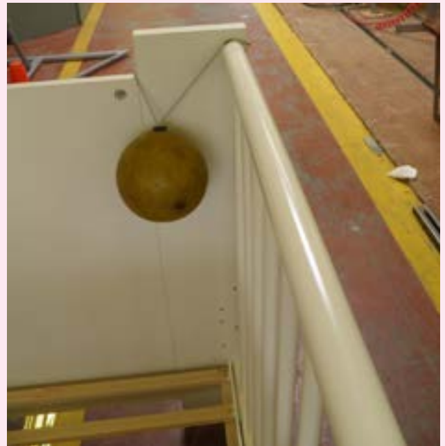
Method of assessing protruding parts of a cot for possibility of entanglement
