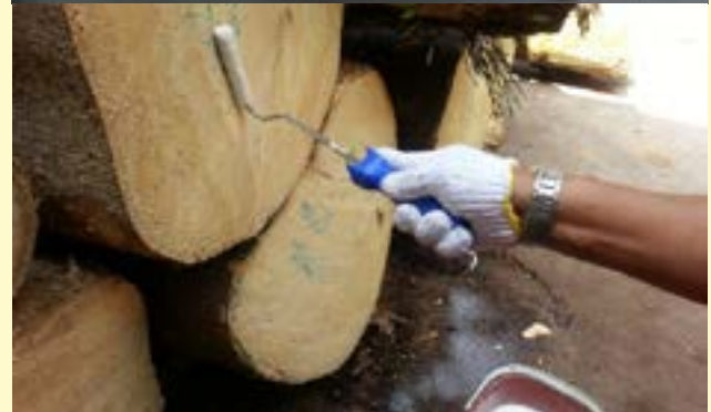
Light coloured timbers (above) like jelutung, sesenduk, rubberwood and pulai should be processed immediately, stacked and dried to avoid attack by the staining fungi. Application of anti-sapstain fungi solutions like boron compound may be necessary for temporary protection (below)
