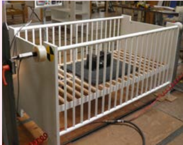
Durability test for baby cot
