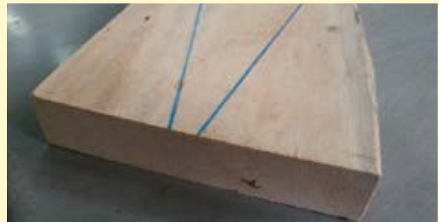
Small pin-holes are common characteristic of defect in cengal. The holes are caused by ambrosia beetles boring into living trees. These beetles die when timber is seasoned
