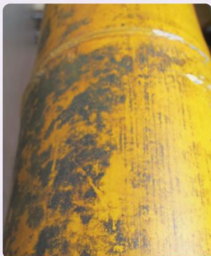
Mold growing on the surface of bamboo
