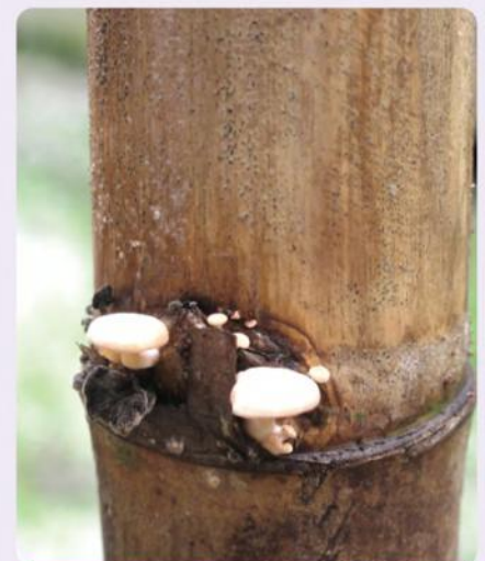
Fungi fruiting bodies on bamboo showing advanced stage of decay
