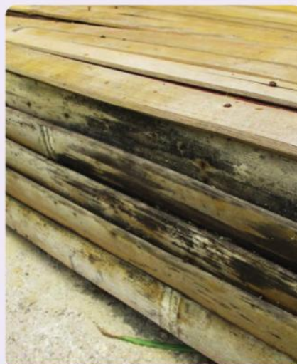
Decayed bamboo strips exposed to outdoor condition
