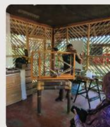
Making bicycle frame using bamboo
