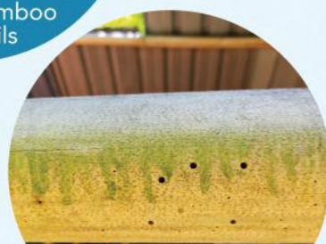
Borer attack on bamboo bar
