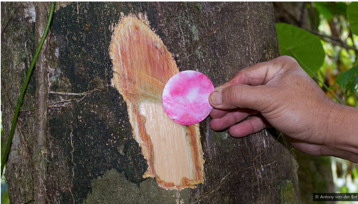
A quick in-situ test is to use detector paper that turns pink on the spot (Credit: Antony van der Ent)
